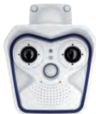
M16 with two MX sensor modules (Day/Night/LPF)
