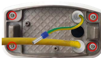
Fig. 12: Installed and ready for Connector Box LSA
